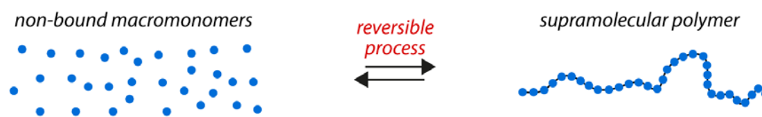
Figure 1. The assembly of monomers that carry suitable non-covalent interactions gives rise to supramolecular polymers. The reversible and dynamic linkage in such materials directly translates into stimuli-responsive properties in the bulk.
